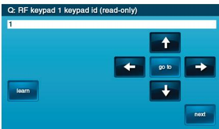
Press the "Learn" button on the CP1-900 panel and the "pair with panel" button on the TS1 to initiate the learning process. The screen will display "Pair with TS1. Initiating learning process." Both the TS1 and CP1-900 panel will display "The learn operation succeeded" when the learning is complete.
